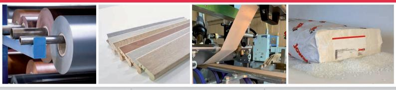
Unfilled PO hot melt adhesives for profile wrapping
