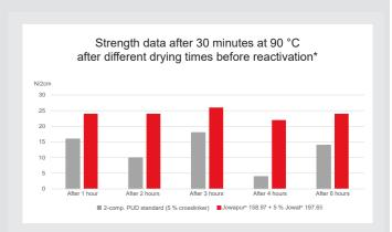
\* The results are based on a series of tests under laboratory conditions. Testing was carried out with a 120 µm film applied onto ABS. The final strengths were determined after a crosslinking time of 7 days and then subject to the heat resistance test mentioned above.
