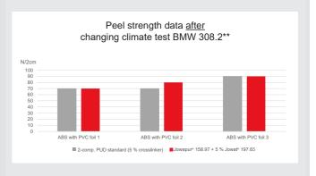
\*\* The results are based on a series of tests under laboratory conditions. The application amount was 50 - 60 g/m² dry (by spraying). Testing was carried out with ABS substrates and three different PVC foils (containing different plasticisers). The exact test cycles of the changing climate test BMW 308.2 are available upon request.
