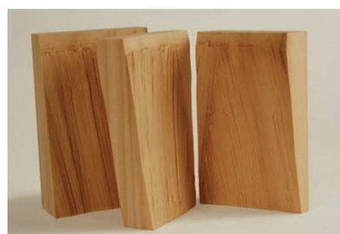
after splitting ... 100 % wood failure.
