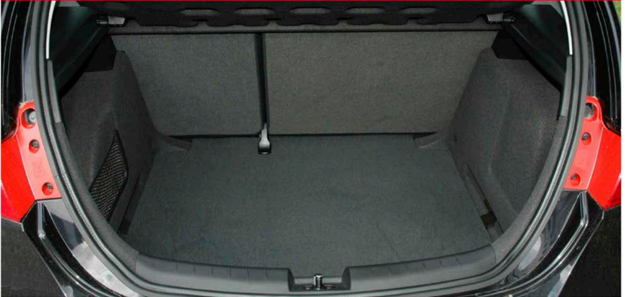
In the automotive industry, trunks are of major significance. Not only are they helpful for transporting groceries, baggage and other items, trunks are also a car compartment where weight reduction plays an essential role. To meet the requirements for a lightweight construction, modern trunk floors are increasingly manufactured from a honeycomb board foamed with polyurethane (PU). Compared to the wood-based materials used in the past, these boards weigh less and are extremely stable.
